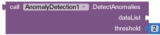
(a) The code block enabling learners to detect anomalies in their dataset of choice based on the Z-Score algorithm integrated into their mobile app.
