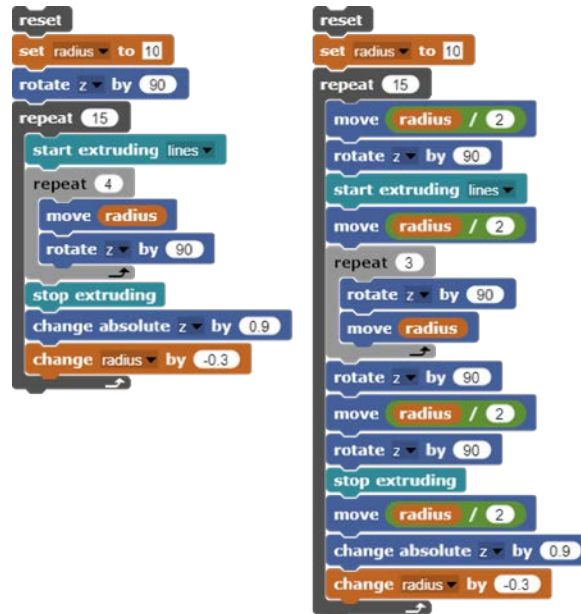
Figure 15. Source code of the leaning tower (left) and its symmetrical counterpart, which has been constructed finding the center with simple geometry (right)
