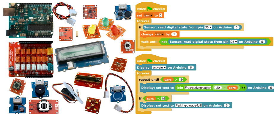
Fig. 1. Arduino Uno Wifi with Tinkerkit and Grove components and IoT-Snap scripts.
